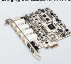
and adding features such as a Hi-Z instrument input for electric guitars and optical S/PDIF I/O, makes MAYA44 XTe a modern and extremly affordable audio interface. The PCIe audio interface is bundled with Cubase LE 5 from Steinberg and compatible with Windows XP. Windows Vista and of course Windows 7 (32-bit and 64-bit supported).
