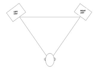
The height of the units, more precisely the top of the woofer, is recommended to be at the ear level of the listener. Keep in mind that in a typical monitoring environment, you are sitting in front of your workstation. Refer to the following diagram:
