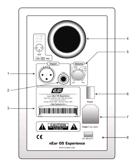
**1. XLR input** – this connector accepts balanced XLR input connections. The signal of the XLR input is mixed together with the TRS input signal through a balanced input amplifier. The XLR input is wired like this:
