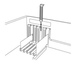
Next, put the Waveterminal 192M PCI card into the slot and make sure it is placed in the slot correctly. The card will fit into your slot and then tighten the screw.
