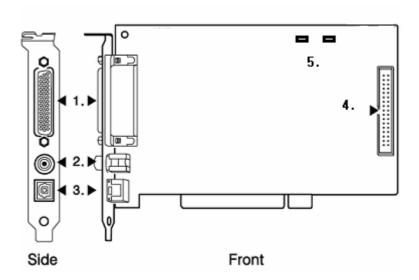
1. D-Sub connector: Connect Waveterminal 192M PCI card with the break out box.
