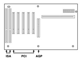
There are 3 kinds of slots in most of recent computers. The PCI slot is most common and is used for different types of devices from the soundcard to the modem. Usually, the PCI slot is the white-colored slot. The ISA slot is used in older computers and it is marked with a black slot. The AGP slot is only for the video card and is the most recent type of slot. It is marked with a brown slot and is located close to the CPU. It will be not too hard to find the PCI slot for Waveterminal 192M.
