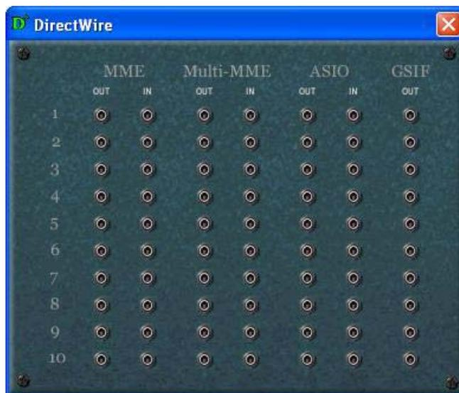
As you can see, MME, Multi-MME, ASIO and GSIF indicate driver names of WaMi Rack 192 Series. Along the vertical channel indicate number, output and input ports of each driver are showed.
