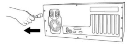
Remove the computer cover. Make sure that you have an available PCI slot in your motherboard to install the MAYA44. Please refer to your computer user's manual to remove the cover.
