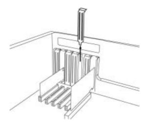
Next, put the MAYA44 PCI card into the slot and make sure it is placed in the slot correctly. The card will fit into your slot and then tighten the screw.
