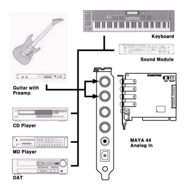
**2. Mic Input (Analog Input 1 &2)** can be used to connect a microphone. A dynamic mic or condenser mic that needs phantom power can also be connected. You can record a voice or musical instruments such as a guitar, bass and piano.
